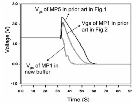
Figure 6. Comparison of the gate-to-source ( $V_{gs}$ ) voltage across some transistors in the proposed I/O buffers and the two previous designs (Fig. 1 and Fig. 2) during the transition from receiving 2.5-V to transmitting 0-V output signals.
