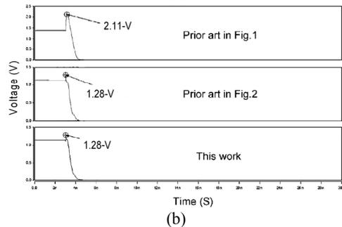
Figure 4. Comparison of the drain-to-source voltage ( $V_{ds}$ ) of (a) MN0 and (b) MN3 between the new proposed I/O buffer and the two previous designs (Fig. 1 and Fig. 2) during the transition from receiving 2.5-V input signal to transmitting 0-V output signal.
