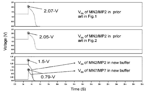
Figure 5. Comparison of the drain-to-source voltage ( $V_{ds}$ ) between transistors in the transmitting circuits during the transition from receiving 2.5-V input signal to transmitting 1.2-V output signal.
