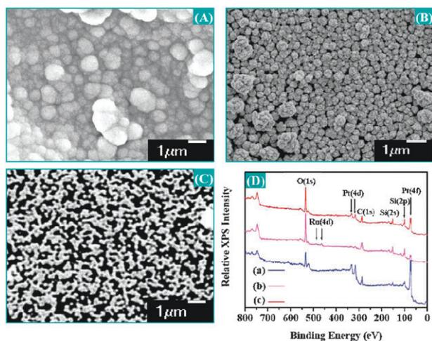
**Fig. 1** SEM images: (A) blanket Pt on flat Si substrate; (B) Ru on blanket Pt; and (C) continuous Pt island network on the flat silicon substrate; (D) X-ray photoelectron spectrum (XPS) of (a) blanket Pt/Si; (b) Ru decorated blanket Pt; and (c) continuous Pt island network.
