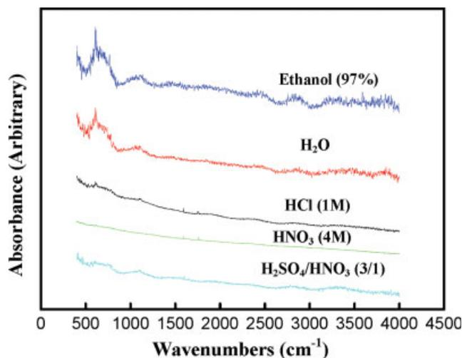
FIG. 1. FTIR spectras of CNTs immersed in different solutions. [Color figure can be viewed in the online issue, which is available at [www.interscience.wiley.com](http://www.interscience.wiley.com).]
