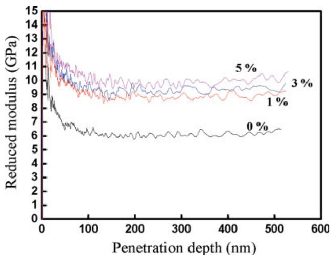
FIG. 4. Reduced modulus versus displacement curves of different CNTs contents on the CNTs/PMMA composite films. [Color figure can be viewed in the online issue, which is available at [www.interscience.wiley.com](http://www.interscience.wiley.com).]
