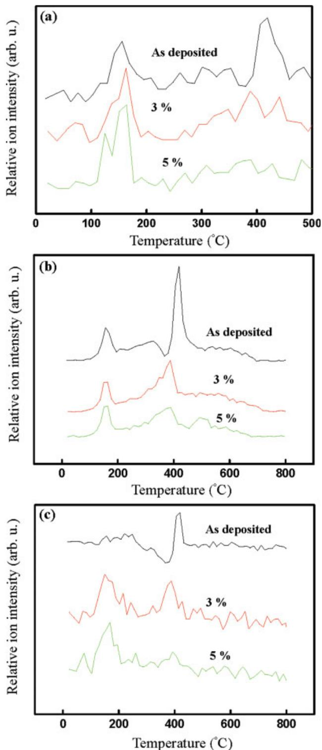
FIG. 7. Production of thermal desorption elements as a function of temperature with different contents of CNTs. (a)  $\text{CH}_3$  ( $m/e = 15$ ), (b)  $\text{CO}_2$  ( $m/e = 44$ ), and (c)  $\text{O}_2$  ( $m/e = 32$ ). [Color figure can be viewed in the online issue, which is available at [www.interscience.wiley.com](http://www.interscience.wiley.com).]
