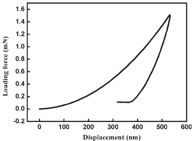
FIG. 3. Typical loading force versus displacement curves obtained from the nanoindenter system.
