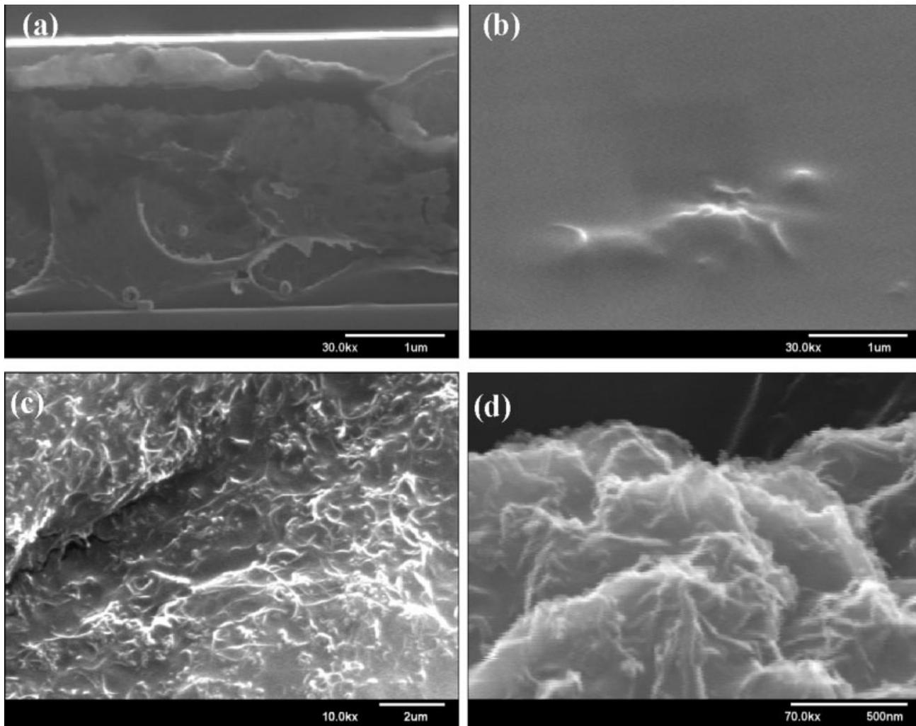
FIG. 2. SEM images of (a) pure PMMA matrix, (b) surface image of MWCNT/PMMA composite, (c) fracture surface image of composite film, (d) large magnitude image of composite film.
