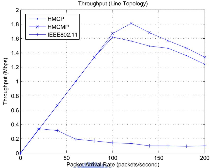
Figure 4.1: The aggregate throughput of a chain topology.
