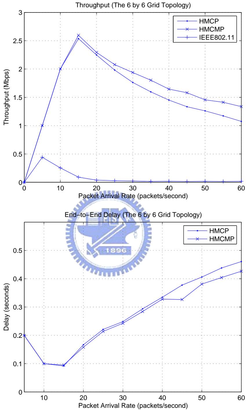
Figure 4.4: The aggregate throughput and the average end-to-end delay of a 6 by 6 grid topology.
