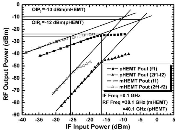
Fig. 5. Measured output performances of pHEMT and mHEMT upconverters. RF = 40.1 GHz and IF = 0.1 GHz for pHEMT while RF = 38.1 GHz and IF = 0.1 GHz for mHEMT.
