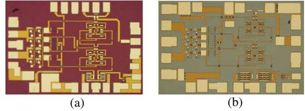
Fig. 3. Micrographs of (a) mHEMT and (b) pHEMT Gilbert upconverters.
