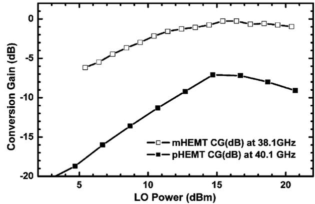
Fig. 4. Measured conversion gain of the pHEMT and mHEMT Gilbert upconverters when the LO frequency is fixed at 20/19 GHz, respectively.
