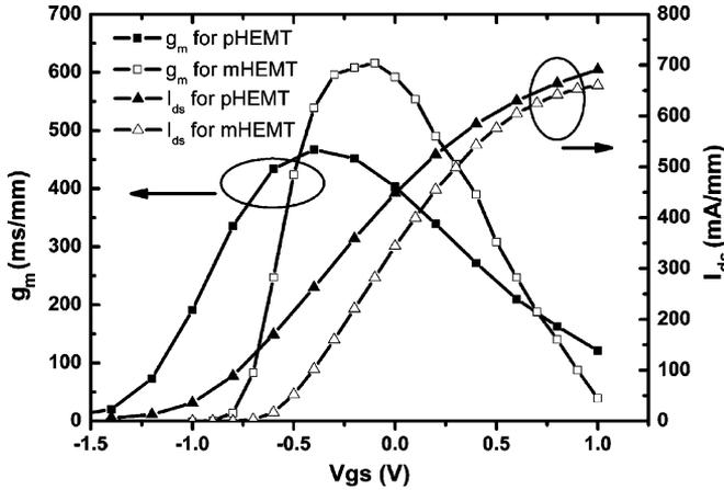
Fig. 1. Measured drain-to-source current ( $I_{ds}$ ) and tranconductance ( $g_m$ ) with respect to gate-to-source voltage for both pHEMT and mHEMT.
