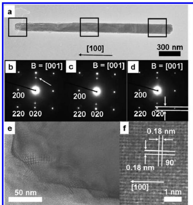
**FIGURE 2.** TEM studies of a Cu nanopillar: (a) low-magnification image; (b–d) SAED patterns of the rectangular marks in part a indicating the tip, middle, and bottom of the nanopillar (from left to right), respectively; (e) enlarged image of the lower half of the tip in part a; (f) HR image of the tip in part a.
