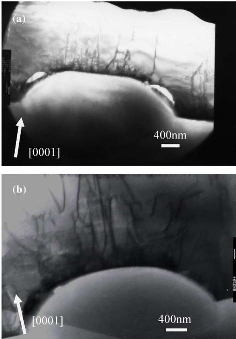
Fig. 2. Cross-section bright-field TEM image of GaN buffer layer grown on (a) MPSS and (b) HPSS. The images were taken on  $\langle 11 - 20 \rangle$  zone axis.
