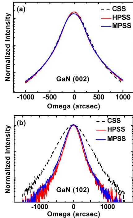
Fig. 3. Rocking curves of the GaN films grown on CSS, MPSS, and HPSS. (a) (002) plane, (b) (102) plane.
