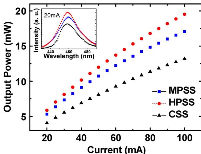
Fig. 4. Light-output power characteristics of 460-nm InGaN-based LEDs grown on CSS, MPSS, and HPSS. The inserted figure shows the EL spectra of the three type LEDs, where the injection current was 20 mA.
