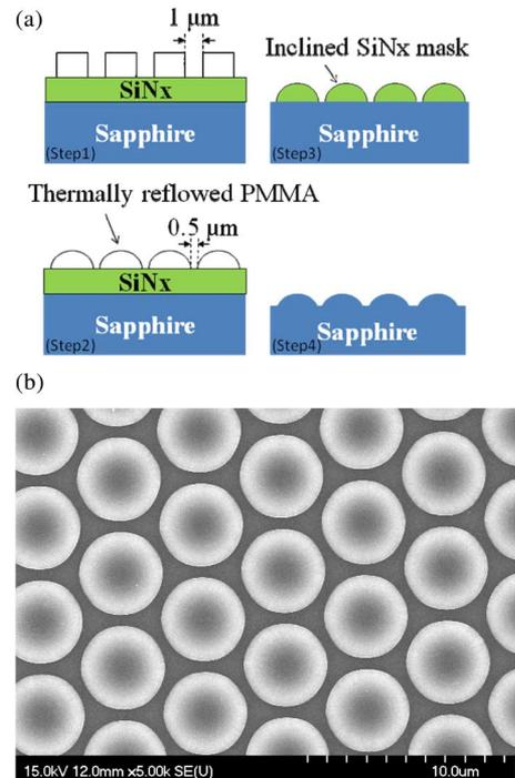
Fig. 1. (a) Process flow of the HPSS with submicrometer spacing. (b) Top-view SEM image of the HPSS. The diameter and the closest spacing between each hemisphere are 4.3 and 0.5 μm, respectively.
