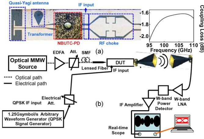
Fig. 1. (a) Top view of the demonstrated device and the simulated frequency response of the coupling loss. (b) Measurement system setup for QPSK wireless data transmission.
