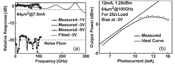
Fig. 2. (a) Measured and fitted O–E frequency responses of the NBUTC-PD. (b) Photogenerated MMW power versus photocurrent of NBUTC-PD
