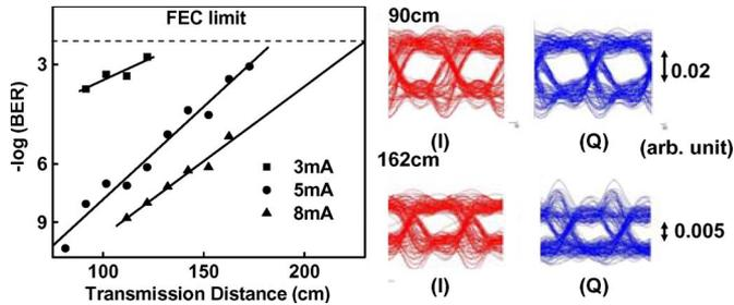
Fig. 5.  $-\log(\text{Bit Error Rate})$  versus transmission distance under different photocurrents during 1.25 billion symbols per second QPSK data transmission. Measured  $I$  and  $Q$  eye patterns under an 8-mA photocurrent at 90 and 162 cm are also specified.
