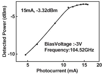
Fig. 4. Detected MMW power versus output photocurrent of our device
