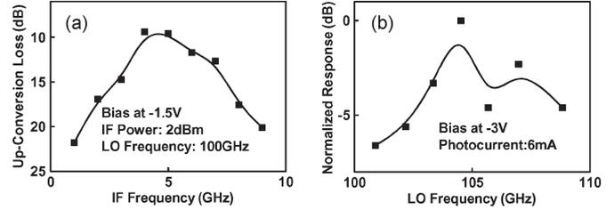
Fig. 3. (a) Frequency response of the up-conversion loss of our QPSK data transmission system measured under a fixed LO frequency (100 GHz) and different IF frequencies. (b) Measured O–E frequency response under different LO frequencies without IF injection.
