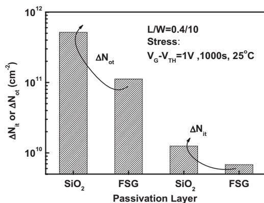
FIG. 6. Stress-induced bulk trap generation ( $\Delta N_{ot}$ ) and interface state generation ( $\Delta N_{it}$ ) for nMOSFETs with FSG and SiO<sub>2</sub> passivation layer at  $V_G - V_{TH} = 1$  V constant voltage stress.
