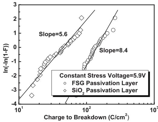
FIG. 5. Weibull plot of charge-to-breakdown distribution for nMOSFETs with FSG and SiO<sub>2</sub> passivation layer at 5.9 V constant voltage stress.
