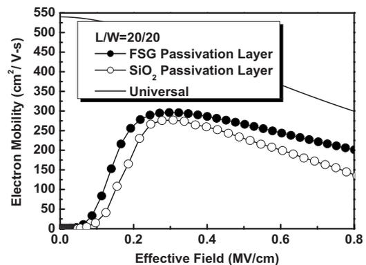
FIG. 4. Electron mobility extracted by split  $C-V$  method for nMOSFETs with FSG and  $\text{SiO}_2$  passivation layer.
