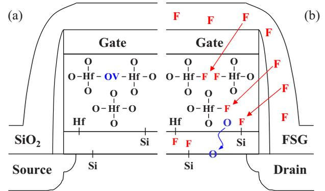
FIG. 3. (Color online) Schematic diagram for the nMOSFET with (a)  $\text{SiO}_2$  and (b) FSG passivation layer. Oxygen vacancy is defined as OV in the figure.
