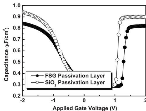
FIG. 2. High frequency  $C-V$  curve for the  $\text{HfO}_2/\text{SiON}$  gate stack with FSG and  $\text{SiO}_2$  passivation layer.
