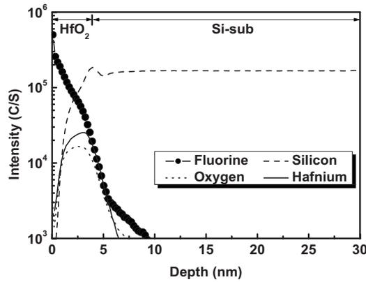
FIG. 1. SIMS depth profile of the FSG passivated  $\text{HfO}_2/\text{SiON}$  gate dielectric.
