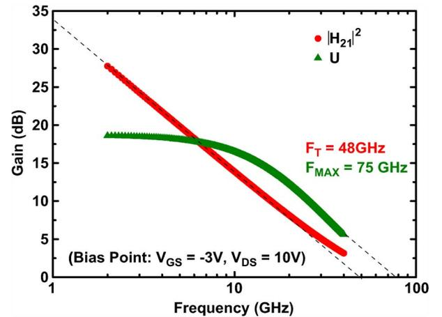
Fig. 3. Intrinsic  $S$ -parameter performance of the device at the bias point of  $V_{GS} = -3\ \text{V}$  and  $V_{DS} = 10\ \text{V}$ .
