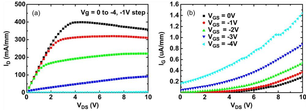
Fig. 2. (a) DC forward characteristics of the 100-nm-gate-recessed n-GaN/AlGaIn/GaN HEMT. The source–drain spacing and device size are  $7\ \mu\text{m}$  and  $2 \times 50\ \mu\text{m}$ , respectively. (b) Gate leakage current density during the device operation.
