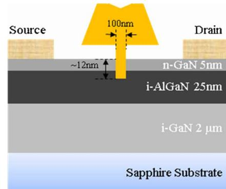
Fig. 1. Cross section of the 100-nm-gate-recessed n-GaN/AlGaIn/GaN HEMT.
