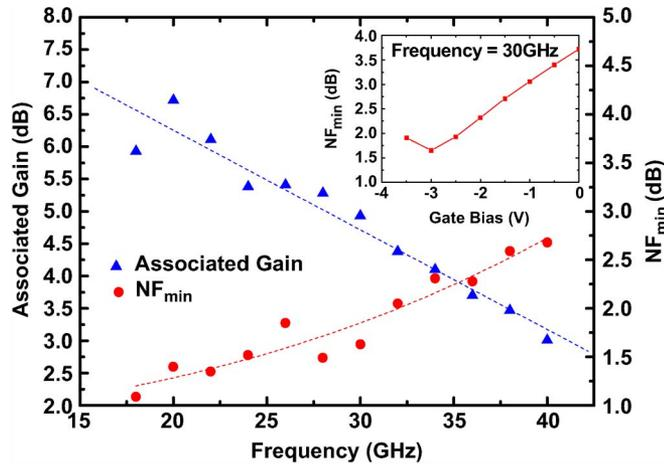
Fig. 4. Frequency dependence of minimum low-noise figure ( $NF_{\min}$ ) and associated gain of the device at the bias point of  $V_{GS} = -3$  V and  $V_{DS} = 10$  V. The inset shows  $NF_{\min}$  against gate bias at  $V_{DS} = 10$  V.
