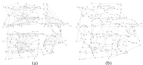
Fig. 12 Experimental result of benchmark s9234. (a) By [18]. The design is partitioned into four clusters and has power saving ratio 19.02%. (b) By our approach. The \beta is set to 0.6 and has power saving ratio 19.30%. It is clear that our approach provides better wiring with the same power saving ratio.
