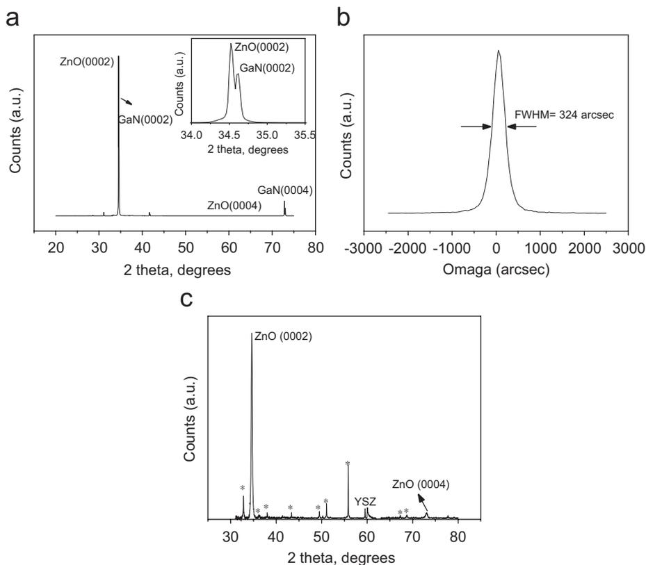
Fig. 1. (a)  $\theta$ - $2\theta$  XRD pattern of ZnO on GaN. The inset is the enlargement of ZnO and GaN (0002) peaks; (b) (0002) rocking curve of ZnO on GaN; (c)  $\theta$ - $2\theta$  XRD pattern of ZnO on YSZ. The peaks marked with \* are reflections from ZnO and YSZ due to the Cu-K $\beta$ , Ni-K $\alpha$  and W-L $\alpha_1$  radiations from a contaminated X-ray source.
