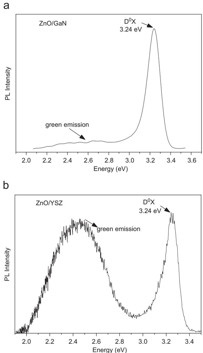
Fig. 3. Room-temperature PL spectra of ZnO layers grown on (a) GaN and (b) YSZ.
