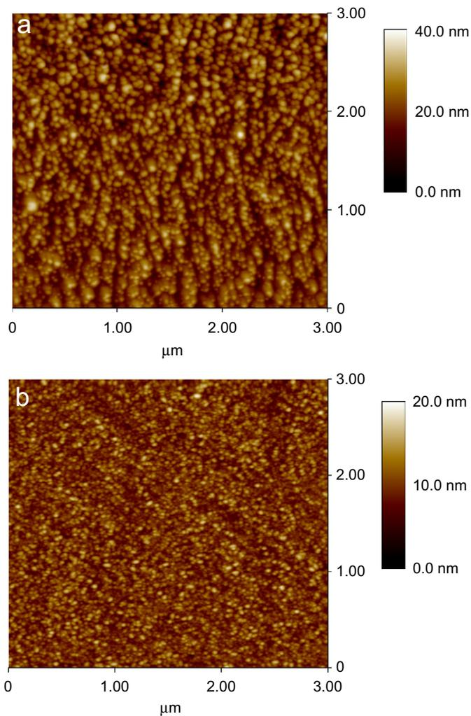
Fig. 2. AFM images of ZnO grown on (a) GaN and (b) YSZ.
