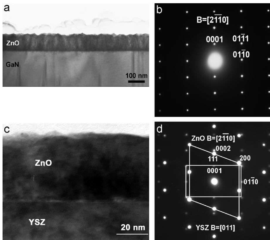
Fig. 4. (a) Cross-sectional bright-field TEM image of ZnO on GaN and (b) the corresponding electron diffraction pattern in  $[2\bar{1}\bar{1}0]$  zone axis. (c) Cross-sectional bright-field TEM image of ZnO on YSZ and (d) the corresponding electron diffraction pattern in  $[1\bar{1}0]$  zone axis of YSZ.
