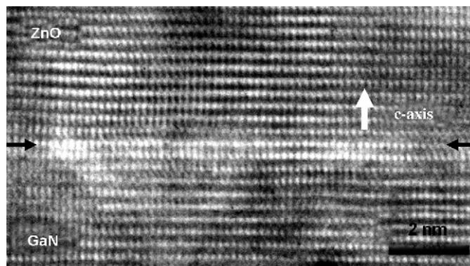
Fig. 5. (a) HRTEM image of the interfacial region between ZnO and GaN viewed along the  $[2\bar{1}\bar{1}0]$  zone axis. The black arrows indicate the position of the interface.
