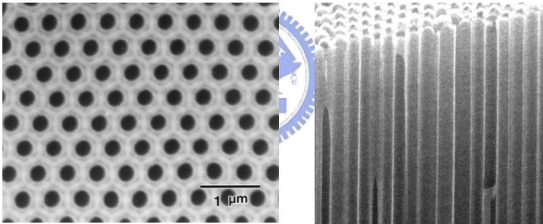
Fig. 1-6. Plane view of AAO<sup>[Masuda-1998-L1340]</sup> Fig. 1-7. Side view of AAO<sup>[Li-2000-131]</sup>
