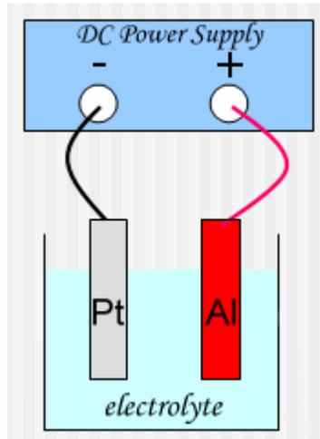
Fig. 1-5 Sketch for AAO fabrication
