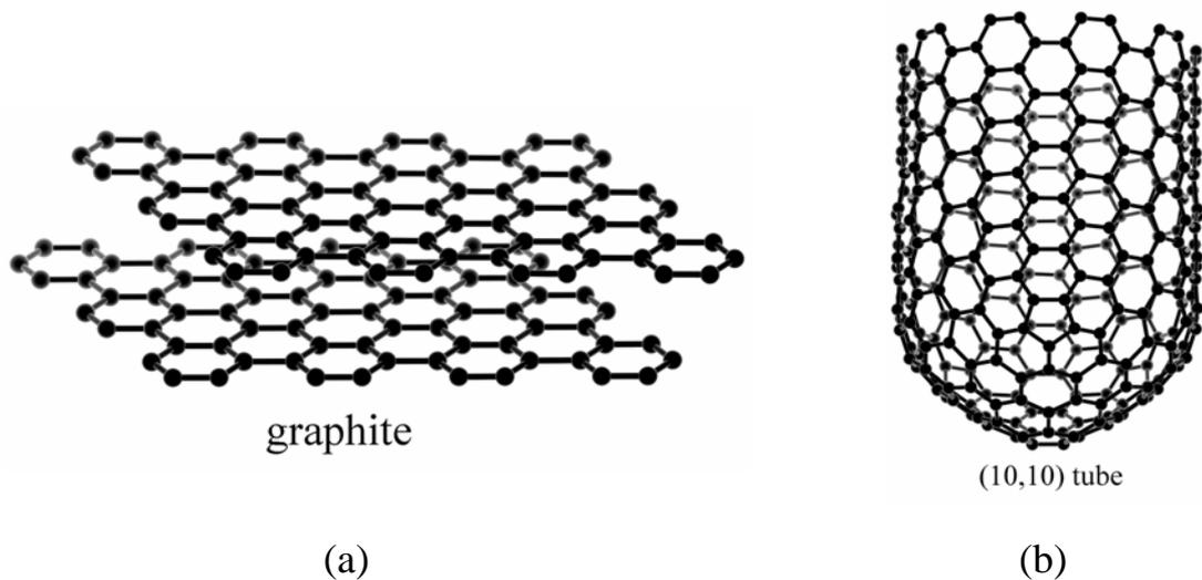
Fig. 1-4. (a) Graphite sheet (b) formed CNT rolled by the graphite sheet.
