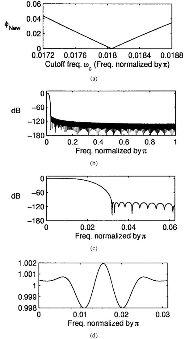
Fig. 2. (a) Objective function  $\phi_{\text{new}}$  versus the cutoff frequency  $\omega_c$ . (b) Magnitude of  $P_0(e^{j\omega})$  (dB). (c) Zoom plot of (b) for the interval  $[0, 2\pi/M]$ . (d) Magnitude of  $T(e^{j\omega})$ . As  $T(e^{j\omega})$  is periodic  $\pi/M$ , only the part in the interval  $[0, \pi/M]$  is shown.
