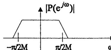
Fig. 1. Typical magnitude response of the prototype for an  $M$ -channel cosine modulated filterbank.
