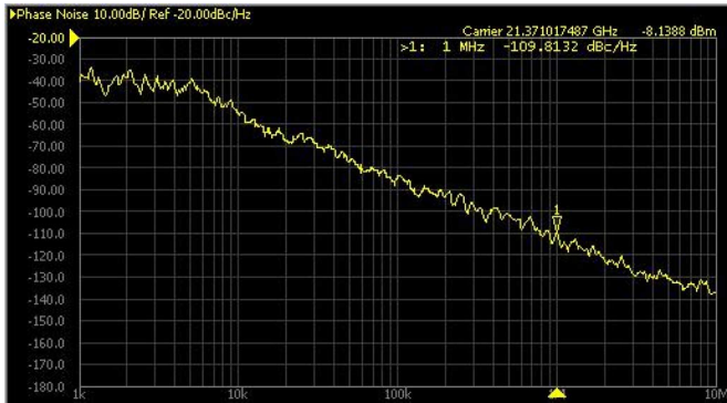
Fig. 6. Measured phase noise of the fabricated VCO at 21.37 GHz with respect to a 1-MHz offset.
