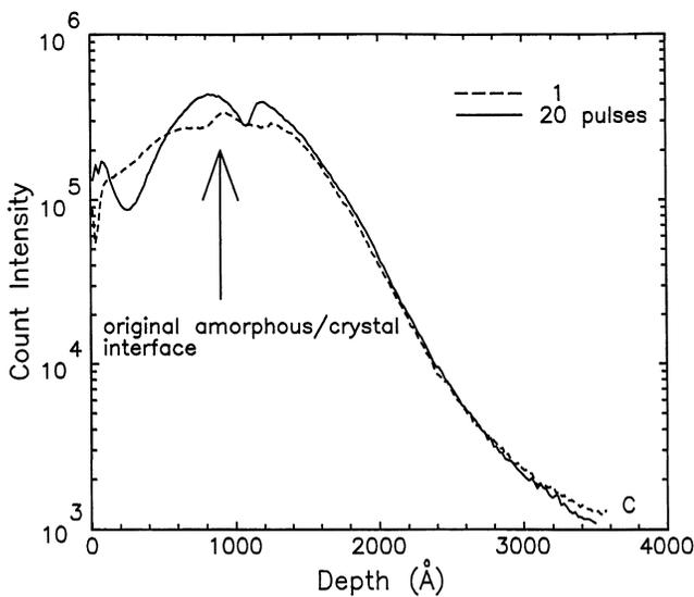
Fig. 7. SIMS depth profiles of C for the  $\text{Si}_{1-x-y}\text{Ge}_x\text{C}_y$  films grown at  $1.0 \text{ J/cm}^2$  for 1 and 20 pulses, respectively.
