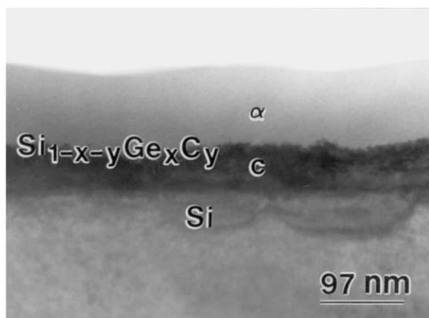
Fig. 1. XTEM image of the as-implanted  $\text{Si}_{1-x}\text{Ge}_x$  film showing the formation of an amorphous  $\text{Si}_{1-x-y}\text{Ge}_x\text{C}_y$  layer.
