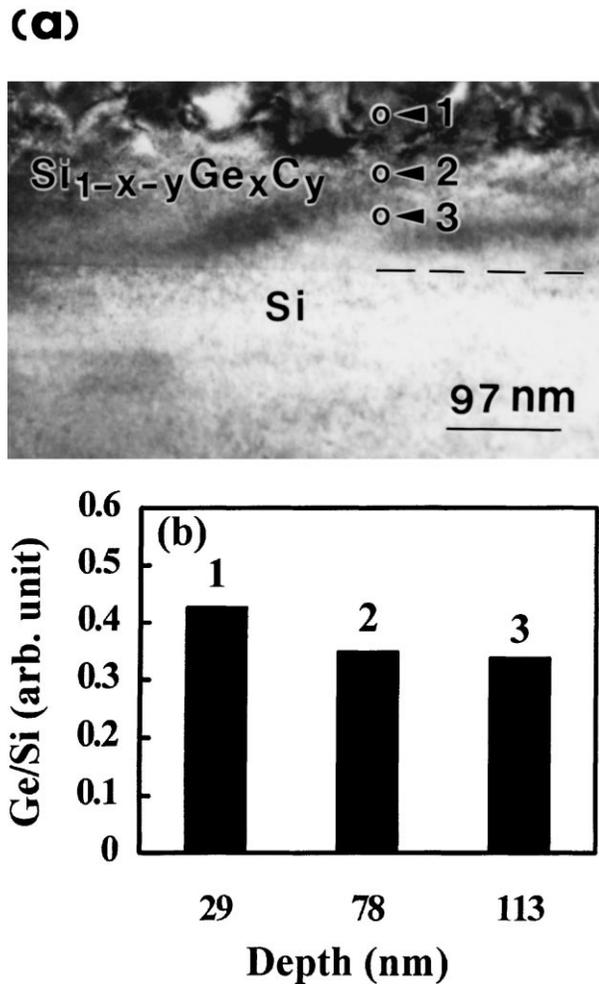
Fig. 3. (a) XTEM image and (b) Ge depth profile of a  $\text{Si}_{1-x-y}\text{Ge}_x\text{C}_y$  film grown at  $1.0 \text{ J/cm}^2$  showing the strong strain contrast and Ge segregation to the film surface. Ge/Si is the atomic concentration ratio,  $x/(1-x)$ , of  $\text{Si}_{1-x}\text{Ge}_x$ . The areas probed by the electron beam for EDS analysis are denoted as '0' and assigned as 1, 2, and 3, respectively.
