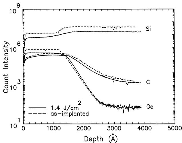
Fig. 4. SIMS depth profiles of Si, Ge, and C for the  $\text{Si}_{1-x-y}\text{Ge}_x\text{C}_y$  film grown at  $1.4 \text{ J/cm}^2$  and the as-implanted  $\text{Si}_{1-x-y}\text{Ge}_x\text{C}_y$  film, respectively.
