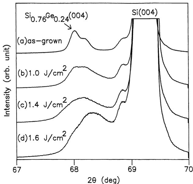
Fig. 9. XRD patterns of (a) the as-grown Si<sub>0.76</sub>Ge<sub>0.24</sub> film, and the Si<sub>0.76</sub>Ge<sub>0.24</sub> films annealed at (b) 1.0, (c) 1.4, and (d) 1.6 J/cm<sup>2</sup>, respectively.
