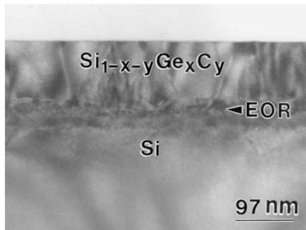
Fig. 2. XTEM image of an epitaxial  $\text{Si}_{1-x-y}\text{Ge}_x\text{C}_y$  film grown at 0.4 J/cm<sup>2</sup>.
