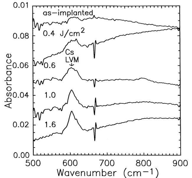
Fig. 5. FTIR absorbance spectra of the as-implanted  $\text{Si}_{1-x-y}\text{Ge}_x\text{C}_y$  film and the epitaxial  $\text{Si}_{1-x-y}\text{Ge}_x\text{C}_y$  films grown at various energy densities.
