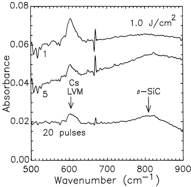
Fig. 6. FTIR absorbance spectra of the epitaxial  $\text{Si}_{1-x-y}\text{Ge}_x\text{C}_y$  films grown at  $1.0 \text{ J/cm}^2$  for various pulse number.
