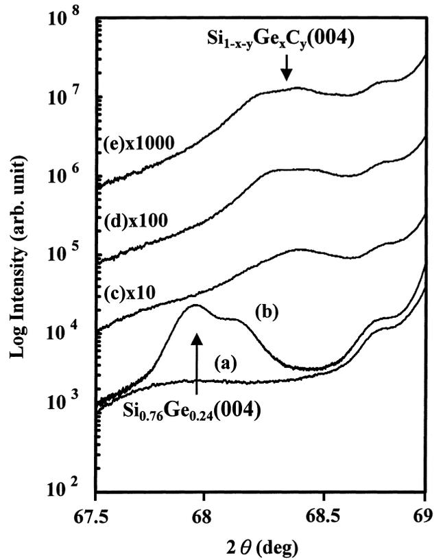
Fig. 8. XRD patterns of (a) the as-implanted  $\text{Si}_{1-x-y}\text{Ge}_x\text{C}_y$  film, (b) the as-grown  $\text{Si}_{0.76}\text{Ge}_{0.24}$  film, and the  $\text{Si}_{1-x-y}\text{Ge}_x\text{C}_y$  films grown at (c) 0.6, (d) 1.0, and (e)  $1.6 \text{ J/cm}^2$ , respectively.
