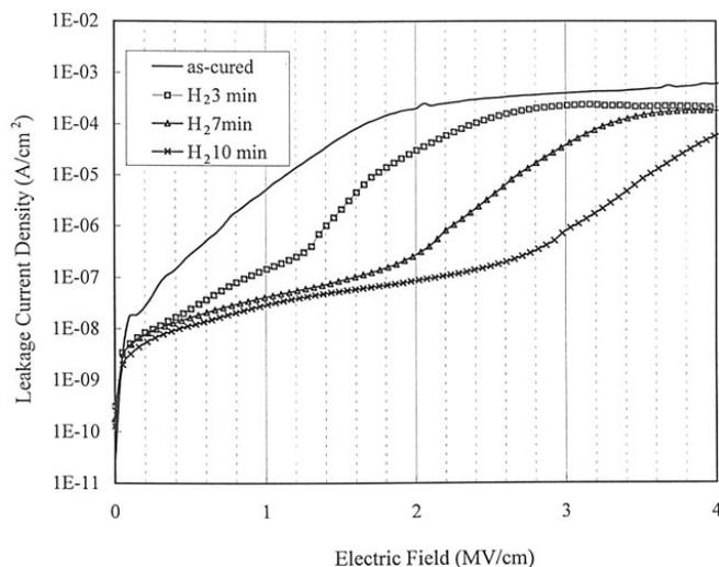
**Figure 5.** The leakage current density of HSQ after (a, top) NH<sub>3</sub> plasma treatment, (b, bottom) H<sub>2</sub> plasma treatment for different exposure times.
