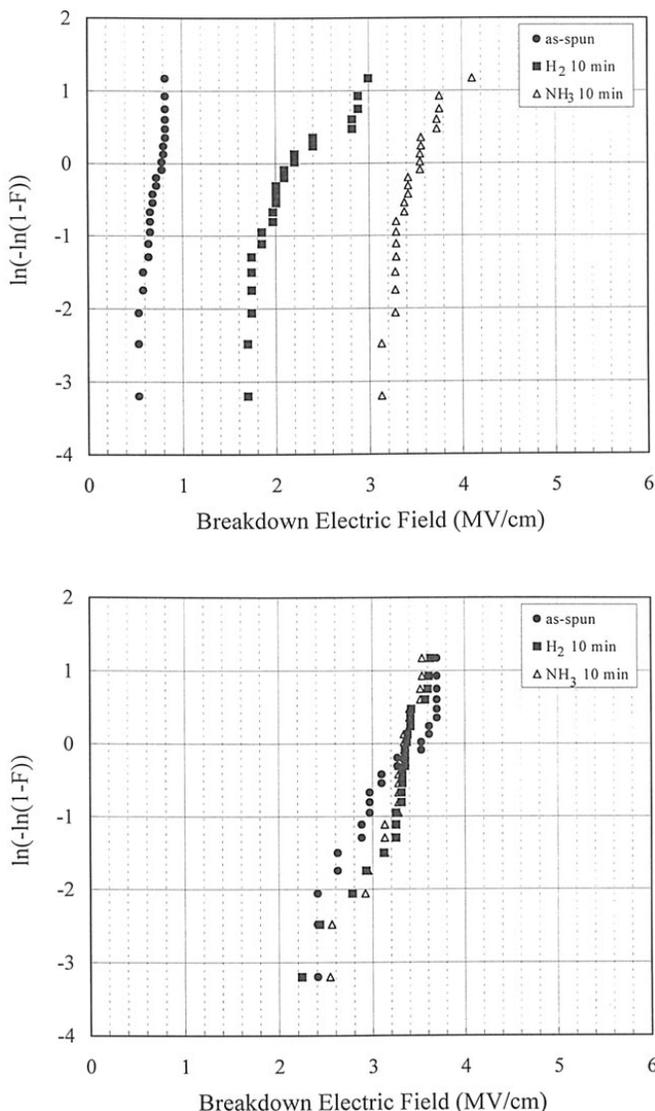
**Figure 7.** Weibull plot of (a, top) Cu/HSQ/Si and (b, bottom) Al/HSQ/Si structures' breakdown electric field ( $E_{BD}$ ) distribution after different plasma treatment conditions.
