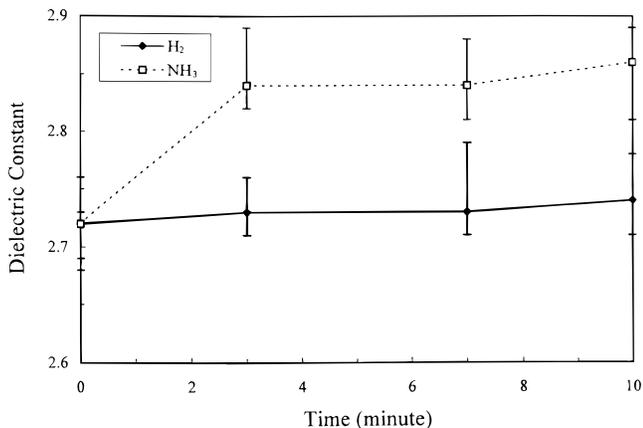
**Figure 2.** The variation of dielectric constant after different plasma treatment conditions.
