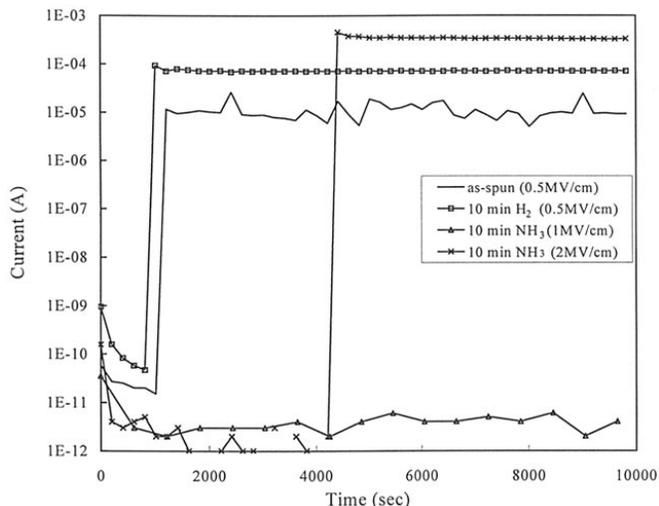
**Figure 8.** Influence of time to failure of Cu/HSQ/Si structure after different plasma treatment conditions.
