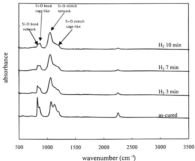
**Figure 1.** FTIR spectra of cured HSQ after (a, top)  $\text{NH}_3$  plasma treatment, (b, bottom)  $\text{H}_2$  plasma treatment for different exposure times.
