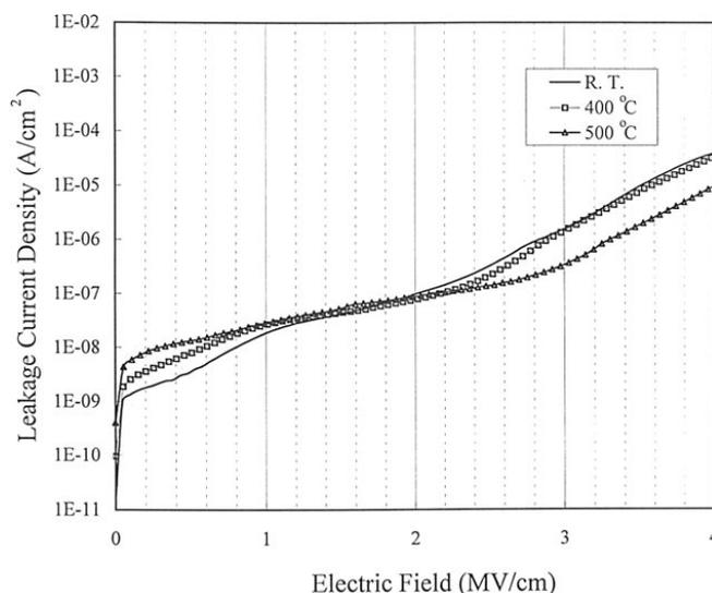
**Figure 6.** The leakage current density of (a, top) as-cured HSQ and (b, bottom) NH<sub>3</sub> plasma-treated HSQ after annealing at 400 and 500°C for 60 min.
