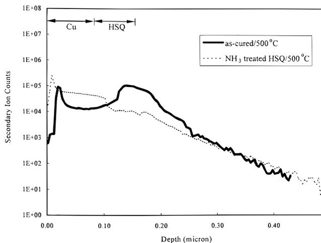
**Figure 3.** (a, top) SIMS depths profile of as-cured HSQ. (b, bottom) Comparing the Cu penetrated into HSQ after annealing at  $500^\circ\text{C}$  for 60 min.
