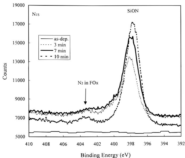
**Figure 4.**  $\text{N}_{1s}$  XPS spectra of HSQ after  $\text{NH}_3$  plasma treatment for different exposure times.
