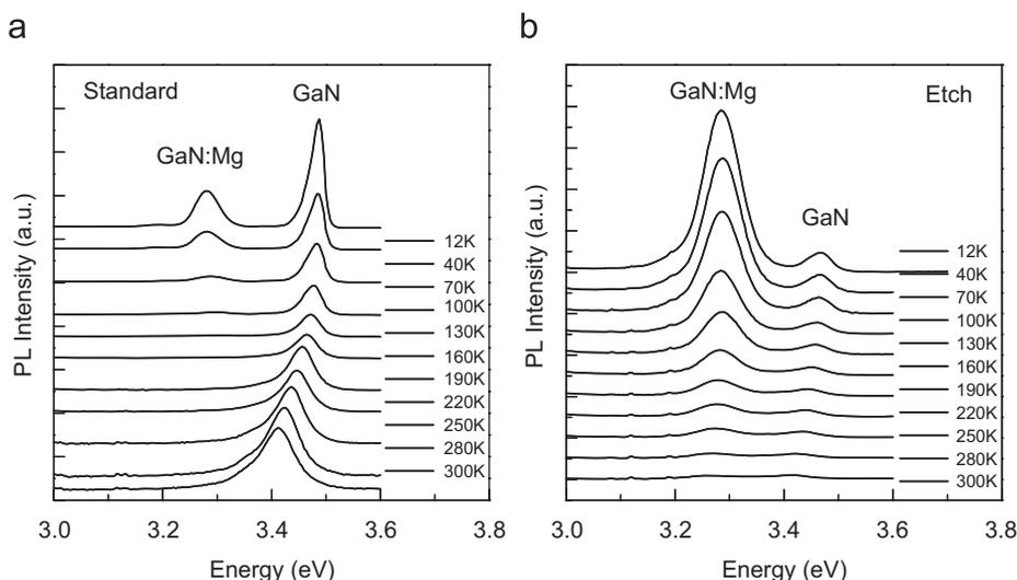
Fig. 3. PL emission spectra of standard (non-etched) and wet-etched LED samples measured at varied temperature.
