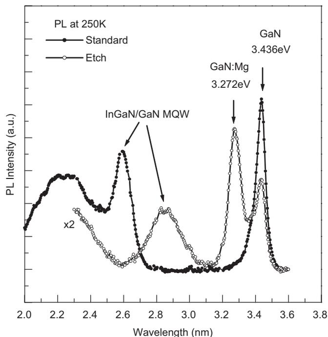
Fig. 4. PL emission spectra of standard (non-etched) and wet-etched LED samples measured at 250 K. The PL emission peaks of InGaN/GaN MQW, GaN:Mg and GaN were both observed.
