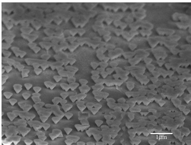
Fig. 1. Self-assembled inverted hexagonal pyramids observed in the mesa region.
