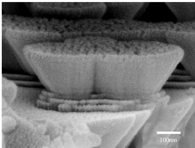
Fig. 2. Self-assembled inverted hexagonal pyramids consisting of the n-type GaN:Si bottom, MQW active layer and top p-type GaN:Mg layer.
