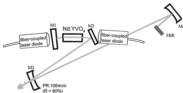
Fig. 2. Configuration of a passively mode-locked Nd:YVO<sub>4</sub> laser with a SBR.
