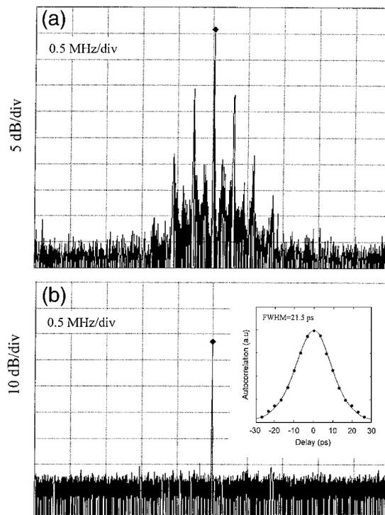
Fig. 3. Power spectrum analyzer signal for the (a) QML and (b) CML states. Autocorrelation of 21.5-ps pulses at 20-W output power is shown in the inset of (b).
