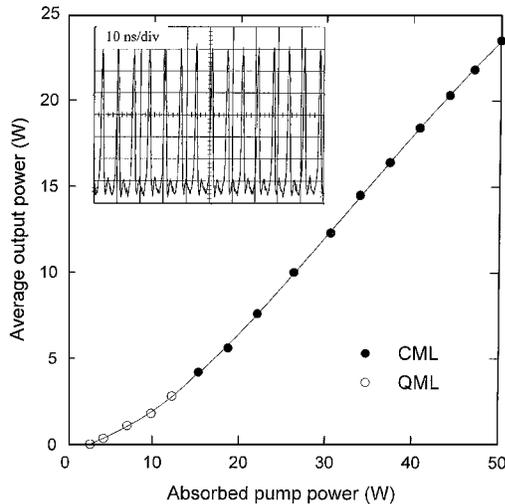
Fig. 4. Dependence of the average output power on the absorbed pump power. Self-starting cw mode locking is obtained for more than 4-W output power.
