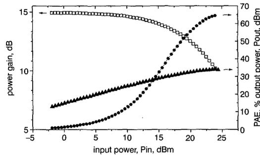
Fig. 2 Power performance of 20 mm E-PHEMT
