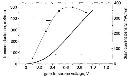
Fig. 1 I-V characteristics of 120  $\mu\text{m}$  E-PHEMT
