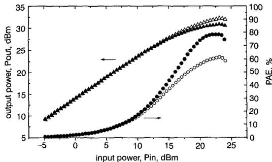
Fig. 3 Power performance of 20 mm E-PHEMT matched for maximum output power and PAE, respectively
