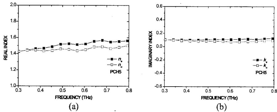
Figure 2. (a) Extraordinary and ordinary indices of refraction of the LC, PCH5, is shown as a function of frequency between 0.2 to 0.8 THz. (b) Imaginary indices of refraction of PCH5 in the same frequency range.
