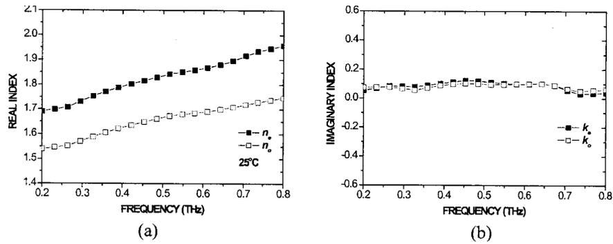
Figure 1. (a) Extraordinary and ordinary indices of refraction of the LC, 5CB, is shown as a function of frequency between 0.2 to 0.8 THz. (b) Imaginary indices of refraction of 5CB in the same frequency range.
