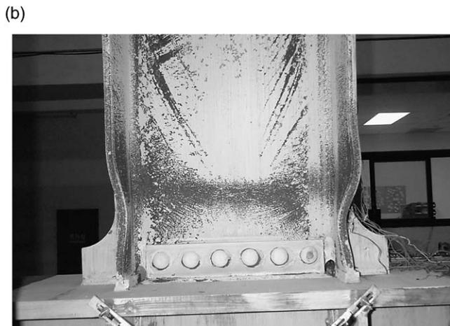
Fig. 7. Yielding and buckling pattern of specimen SRL30 at 3.2% drift.
