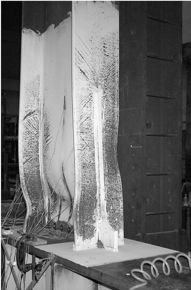
Fig. 10. Local buckling in specimen SRL20 at 3.7% drift.
