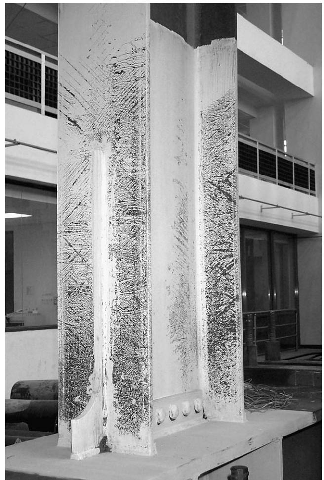
Fig. 9. Formation of beam flange yielding of specimen SRL20 at 2.8% drift.
