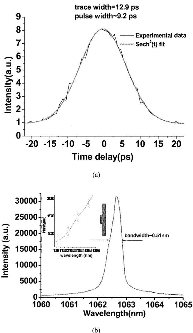
Fig. 3. (a) Envelope of collinear interferometric autocorrelation trace of the mode-locked laser pulses; (b) Corresponding optical spectrum of the laser; inset is the magnification of part of the spectrum, showing minor peaks due to the etalon effect.
