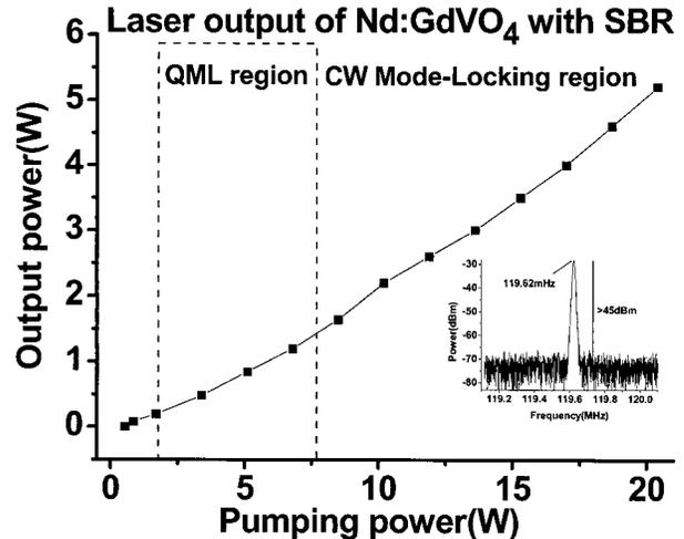
Fig. 2. Dependence of the laser output power on absorbed pump power; inset shows the rf spectrum of the cw mode-locking operation. QML, Q-switched mode locking.
