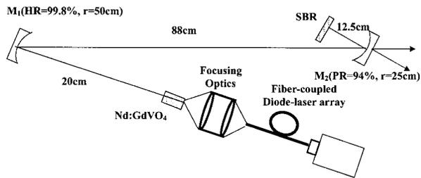
Fig. 1. Cavity configuration of the diode-pumped Nd:GdVO<sub>4</sub> laser. M<sub>1</sub> and M<sub>2</sub>, mirrors; HR, high reflection; PR, partially reflective.
