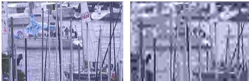
Fig. 16. Frame 15 of the Harbour sequence at 470 kbps (right: original MC-EZBC, left: MC-EZBC with motion information scalability).
