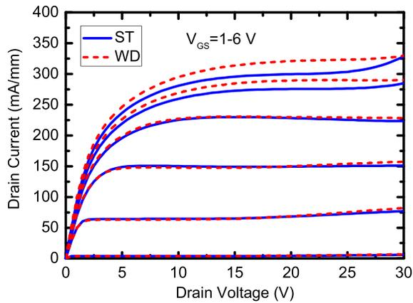
Fig. 2. Output characteristics of LDMOS transistors with wide-drain and standard multifinger structures. The channel width of one finger is  $5 \mu\text{m}$ .
