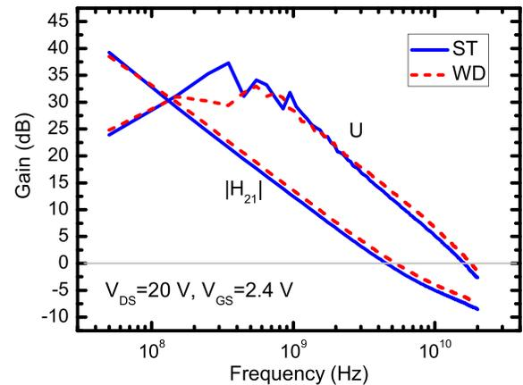
Fig. 4. Short-circuit current gain ( $H_{21}$ ) and unilateral power gain ( $U$ ) of LDMOS transistors with WD and ST multifinger structures. The channel width of one finger is  $5 \mu\text{m}$ .
