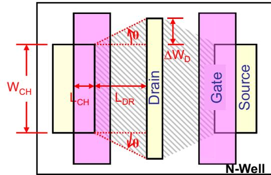
Fig. 1. Layout structure of wide-drain multifinger LDMOS in a unit cell. The drain contact width is larger than the channel width, so the equivalent drift region width is larger than that in conventional devices.
