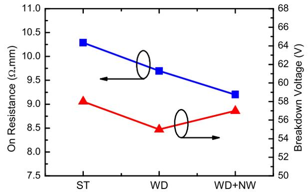
Fig. 3. On-resistances and breakdown voltages of LDMOS transistors with different drain contact and channel widths. ST and WD are the ST and WD devices with  $W_{\text{CH}} = 5 \mu\text{m}$ . WD + NW is the WD device with  $W_{\text{CH}} = 2.5 \mu\text{m}$ .
