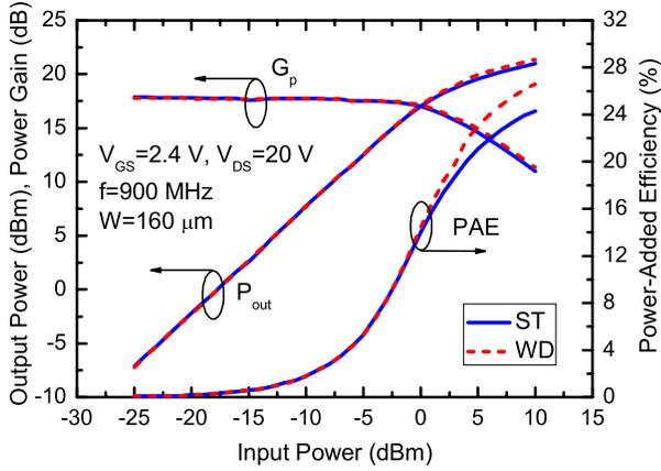
Fig. 5. RF power characteristics of LDMOS transistors with WD and ST multifinger structures. The channel width of one finger is  $5 \mu\text{m}$ .
