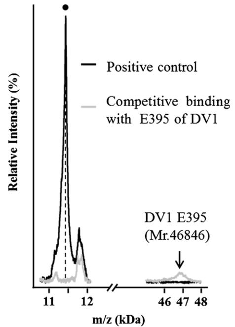
**Fig. 4.** MALDI mass spectra of competitive binding assay. In comparison to the DV1 + anti-E@MBs (black line), the spectra of competitive binding with DV1 E395 (light gray line) showed that MS signal of capsid proteins was reduced and another signal was observed at  $m/z$  46,846, which is that of the DV1 E395 recombinant protein. The circle indicates the MS signal of capsid proteins.
