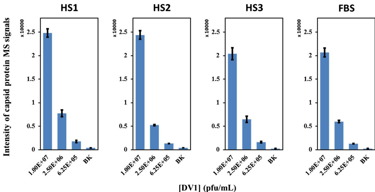
**Fig. 6.** Detection specificity of DV1 in different human sera by MALDI-TOF MS. Different dilutions of DV1 was prepared in three different human sera (HS1–HS3) and in FBS. The HS without DV1 (BK) was used as control. Intensity of bar graphs indicates concentration dependent of capsid protein signal detected by MALDI-TOF MS.
