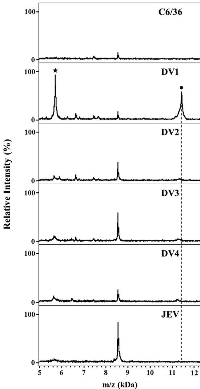
**Fig. 3.** MALDI mass spectra of binding specificity on anti-E@MBs. Two major peaks were detected at  $m/z$  11,431.8 and 5719.5. The circle indicated peak, 11,431.8, corresponds to the single charged ion, and the star indicated peak, 5719.5, corresponds to doubly charged ion.
