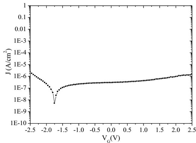
Figure 2. The gate leakage current of the  $\text{La}_2\text{O}_3$  (10nm)/ $\text{HfO}_2$  (5nm) n-InAs MOS capacitor.
