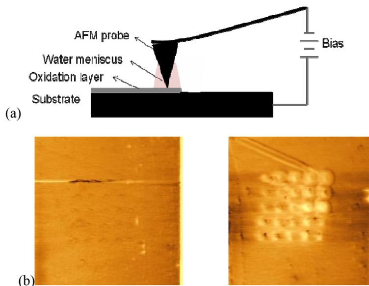
Fig. 1. (a) Schematic of EC-AFM. Applying a bias between the AFM probe and substrate causes a thin layer of oxidation of substrate. The substrate can be metal or doped silicon wafer. The water meniscus is the nanocell for electrochemical reaction. The arrow indicates the moving direction; (b) the patterns in the left image is caused by positive bias for AFM probe as cathode and substrate as anode, whereas the right side image there is no obvious patterns showing while the bias is opposite.
