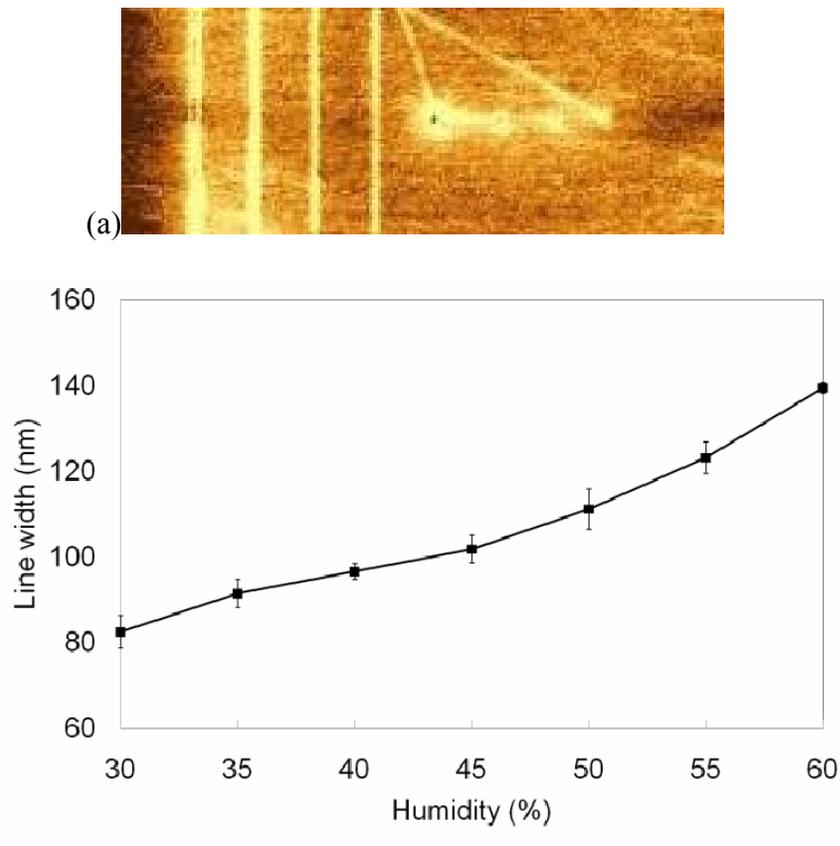
Fig. 2. (a) A set of nanopatterns was designed for evaluating the effect of humidity, and this AFM image was done with humidity of 50% ; (b) width of linear pattern as a function of humidity under the applied bias, 30V. Humidity increases with an interval humidity of 5% from 30% to 60%.
