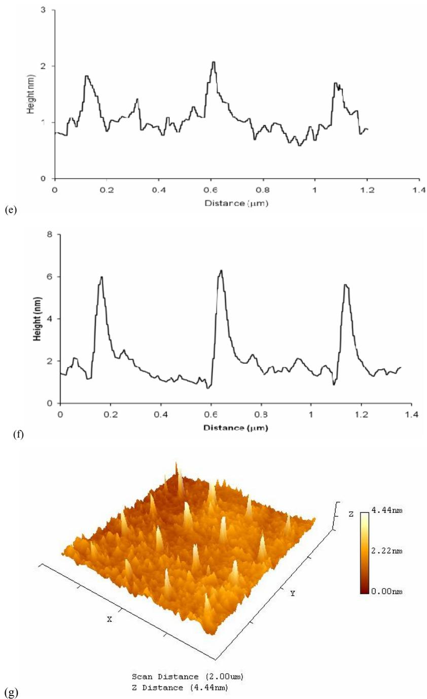
Fig. 3. (a) LFM image of oxide nanodot array; (b) topography of oxide nano-dot array; (c) topography of nano biochip with immobilization of biotin; (d) topography of nano biochip with streptavidin and biotin; (e) the corresponding line profile of (c); (f) the corresponding of line profile of (d); (g) three dimension of AFM image of streptavidin and biotin.
