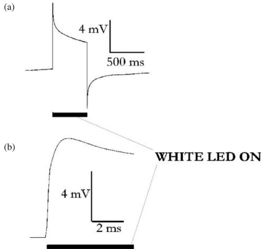
**Fig. 6.** Response value and response time of an isolated 200  $\mu\text{m}$  micro-detector upon radiation with 440 nm light of white LED at an intensity of 400  $\text{mW}/\text{cm}^2$ .
