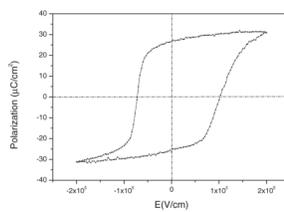
**Fig. 2.** Hysteresis loop measured using the Sawyer–Tower method indicating a remnant polarization of  $25 \mu\text{C}/\text{cm}^2$ , and a value of  $10^5 \text{ V}/\text{cm}$  for the coercive field.
