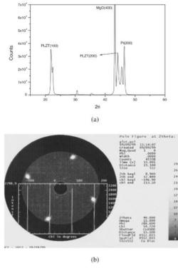
**Fig. 1.** (a) An X-ray diffraction  $2\theta$  spectrum of a PLZT/Pt/MgO heterostructure microdetector indicating (100) atomic ordering of the PLZT active oxide layer grown on (100) ordered Pt, and (b) Pole figure from PLZT/Pt/MgO heterostructure confirming the planar 4-fold symmetry of PLZT film structure.
