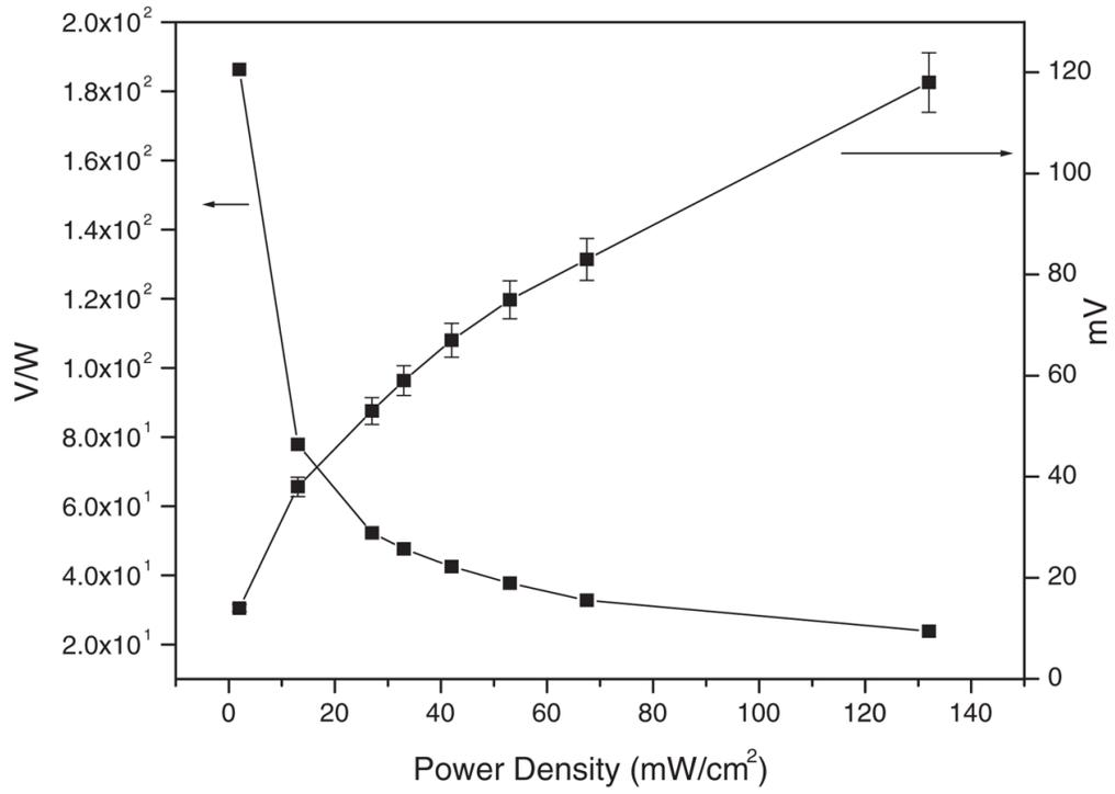
**Fig. 4.** Photovoltaic output, and the responsivity of a 500  $\mu\text{m}$  diameter thin film microdetector as a function of intensity of a solar simulator source.
