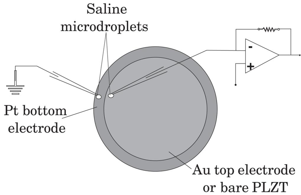
**Fig. 5.** Schematic drawing of the patch-clamp set-up for optical output measurement of an isolated microdetector.
