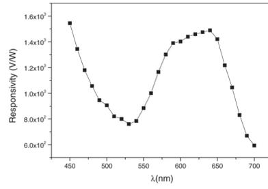
**Fig. 3.** Spectral response of a 500 μm diameter PLZT micro-detector using a xenon lamp with monochromator output set at ~5 mW/cm<sup>2</sup>.
