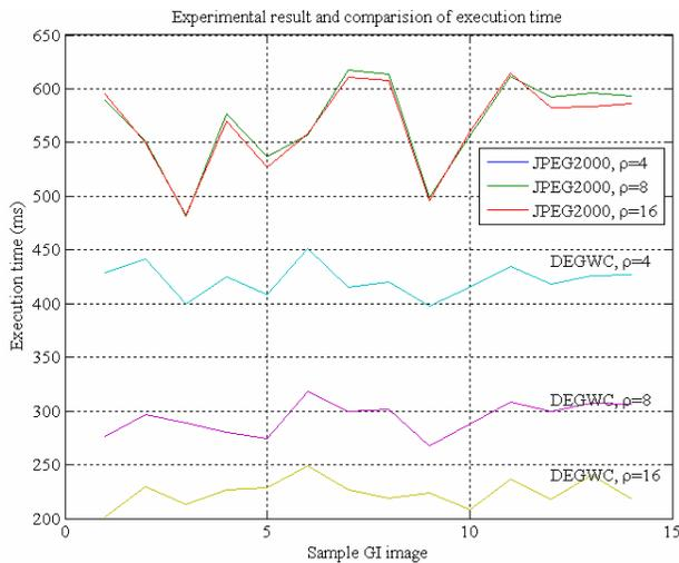
Fig. 5. Comparison of execution times between DEWC and JPEG 2000
