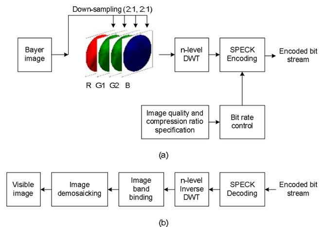
Fig.1 Block diagrams of wavelet-based image compression: (a) image encoder; (b) image decoder.
