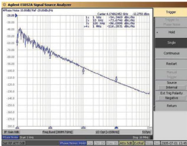
**Figure 4** Phase noise spectrum of the superharmonic-coupled SiGe HBT QVCO. The phase noise is  $-116$  dBc/Hz at 1 MHz offset frequency when the oscillation frequency is 4.17 GHz. [Color figure can be viewed in the online issue, which is available at [www.interscience.wiley.com](http://www.interscience.wiley.com)]
