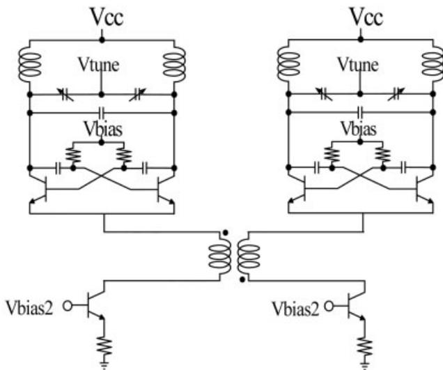
**Figure 1** Schematic of the superharmonic coupled SiGe HBT QVCO
