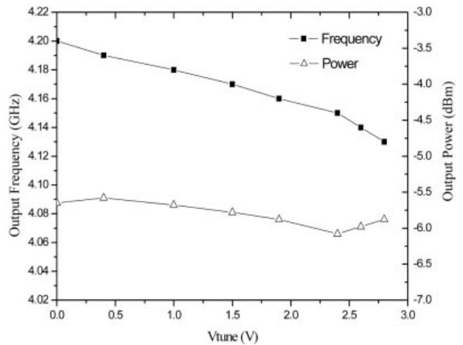
**Figure 3** Output power and frequency as a function of the tuning voltage for the superharmonic-coupled SiGe HBT QVCO
