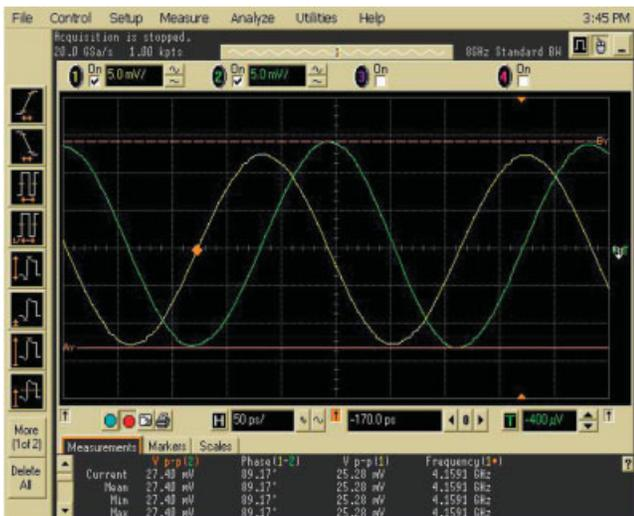
**Figure 5** Time-domain I/Q channel waveforms of the superharmonic-coupled SiGe HBT QVCO. [Color figure can be viewed in the online issue, which is available at [www.interscience.wiley.com](http://www.interscience.wiley.com)]
