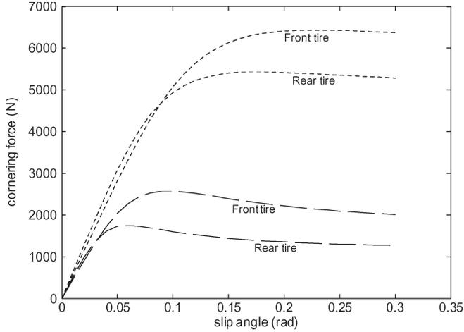
Fig. 2. Cornering characteristics of front and rear tires. Dotted line: high-friction road, and dashed line: low-friction road.
