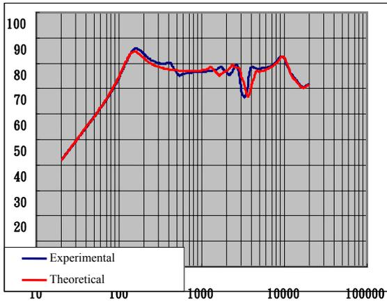
Fig. 7 Theoretical and experimental SPL curves of foam panel
