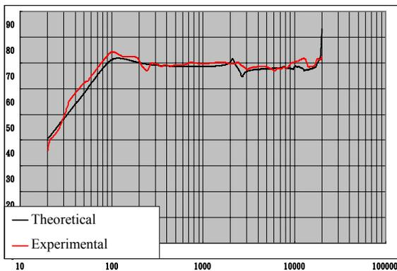
Fig. 8 Theoretical and experimental SPL curves of composite sandwich panel
