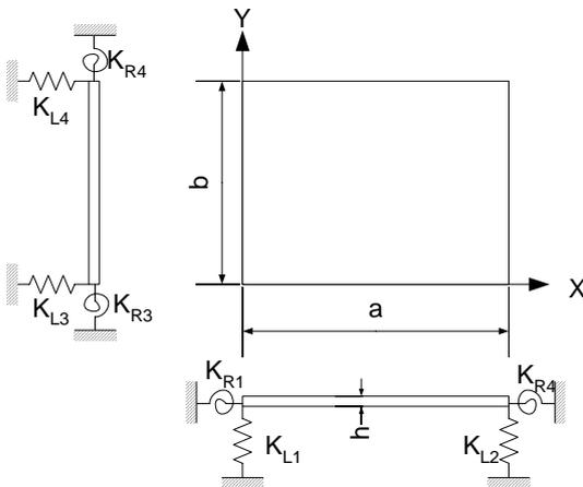
Fig. 2 Mathematical model of flat-panel speaker
