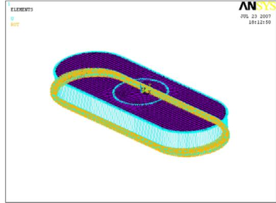
Fig. 4 Finite element model of sound radiator
